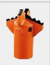
SEA - Star Cut: For drilling in soft ground conditions, the SEA "Star-Cut" drill bit gives high performance and durability. This crosscut type bit has hardened blades with the flushing hole situated behind the cutting edge for optimum grout delivery. Ideal for applications in the following conditions: Sand, Clay and Loose Ground.
